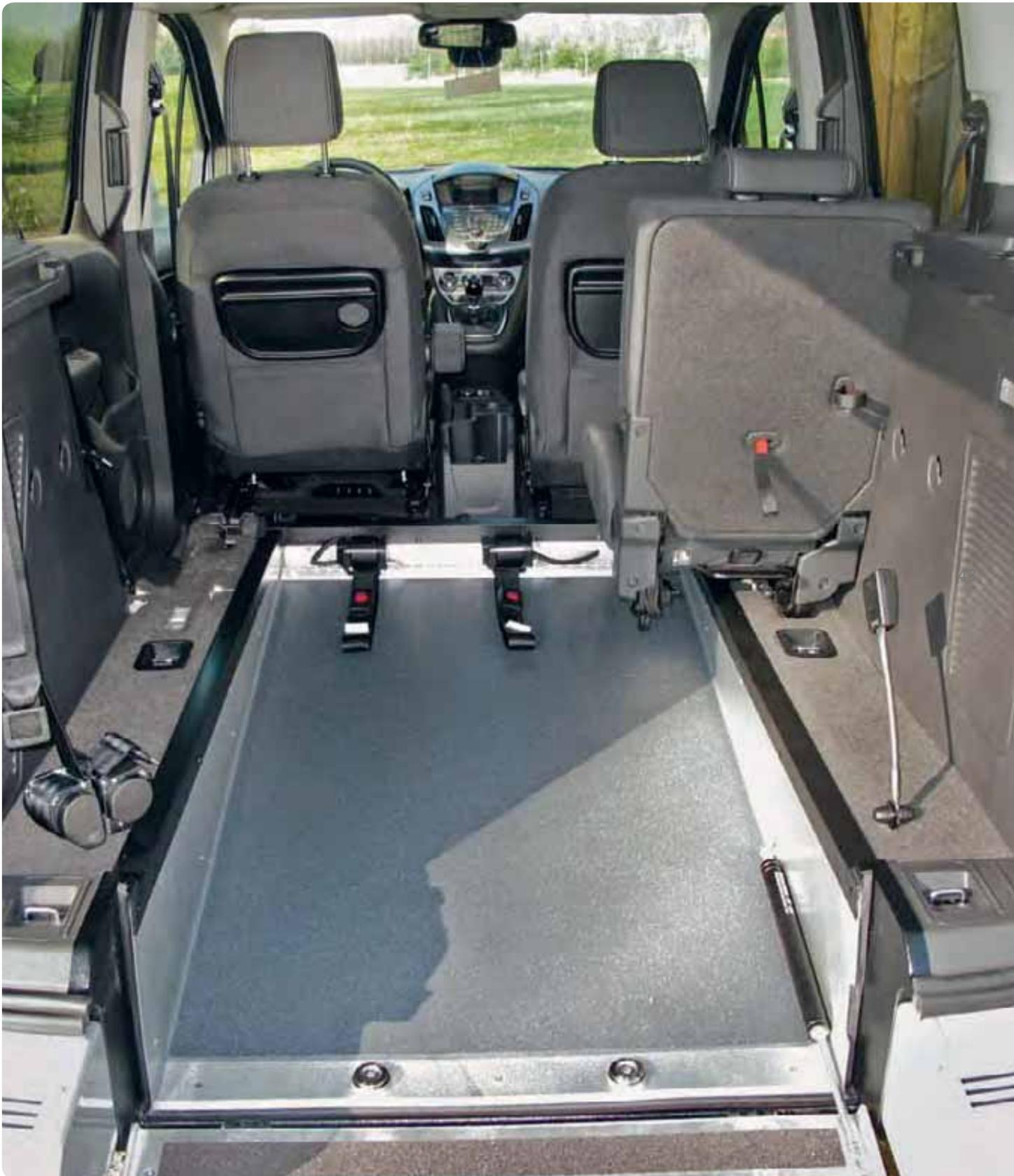
In comparison with other converted vehicles, the impressive cargo area alone makes the Grand Tourneo Connect a very suitable vehicle for wheelchair users. In just a few manual steps, the flexible second row of seats can be very easily converted into a three-seater with space for a wheelchair.
