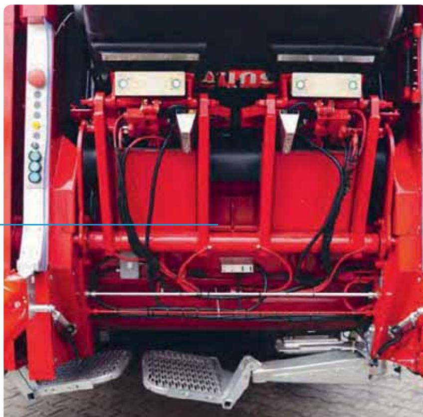
*MEDIUM XLS Split with footboards that can be pneumatically extended and retracted*
