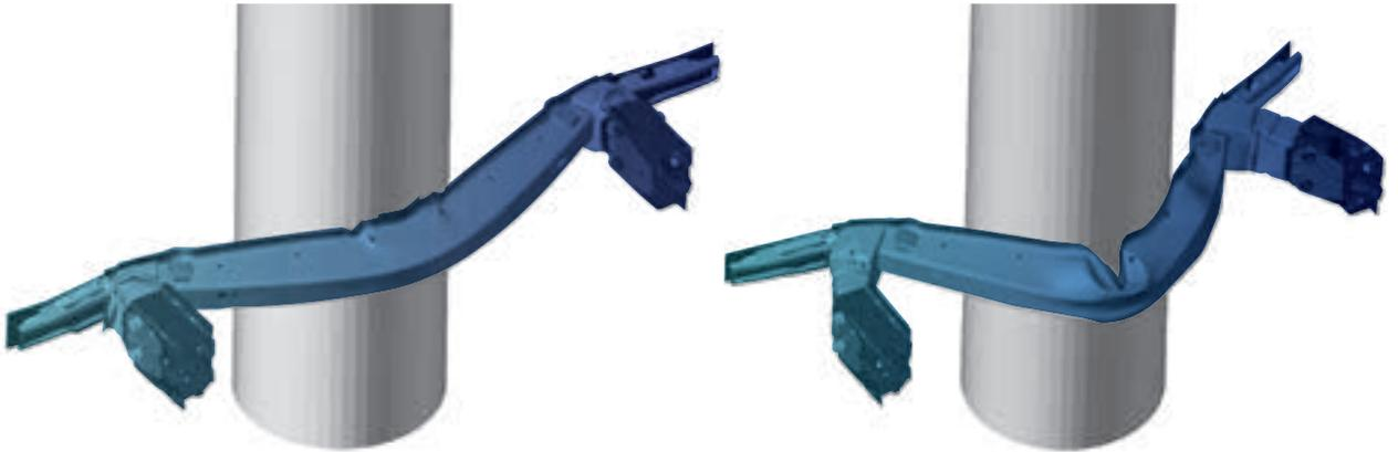
Protection of the battery comes by rigidity or flexible crash management systems for the greatest possible delay in a crash. Which variant is used, depends on the load path concept, i.e. the design of the body-in-white structure with regard to passive safety.
