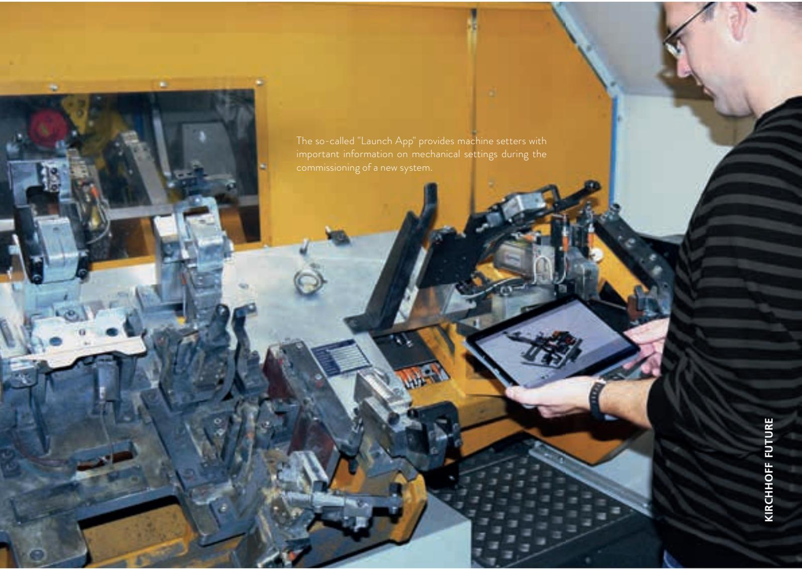
The so-called "Launch App" provides machine setters with important information on mechanical settings during the commissioning of a new system.
