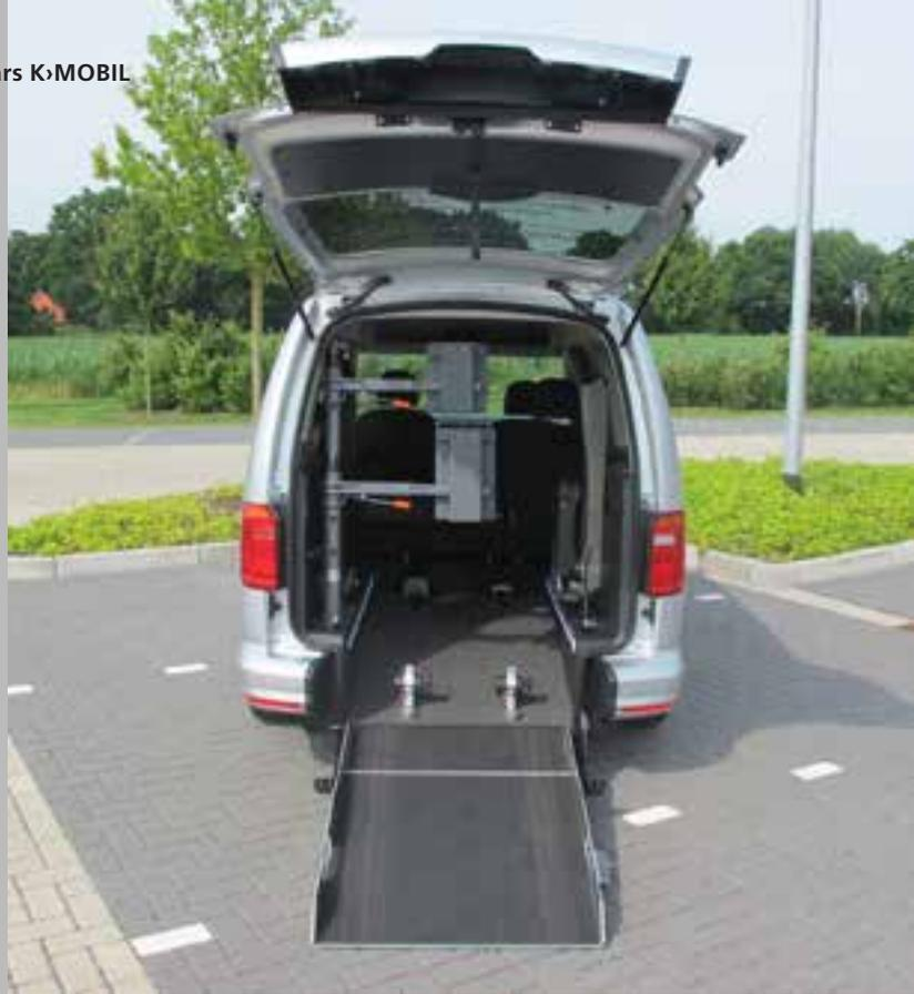
One of the core products of KIRCHHOFF Mobility: The NIVO rear cut-out kit, displayed here in the VW Caddy. Disability-access conversions for various high roof station wagon models are based on this kit.
