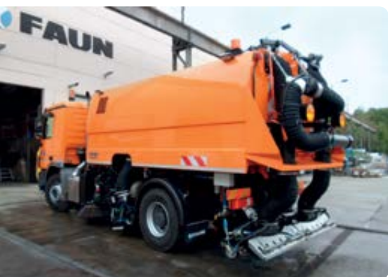
Larger suction and blower hoses and a rear suction system for more power
