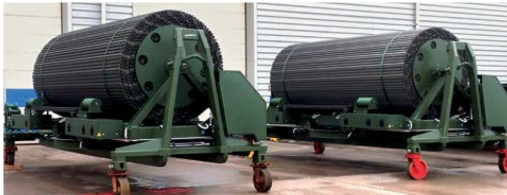
Left: SPOOLRACK units as part of the Heavy Ground Mobility System Right: TRACKRACK units as part of the Heavy Ground Mobility System
