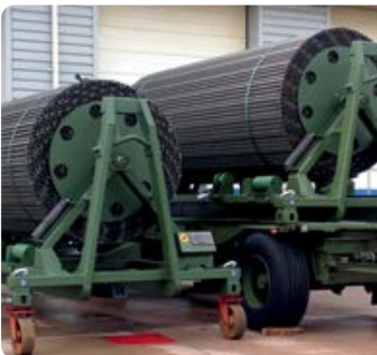
Left: SPOOLRACK units as part of the Heavy Ground Mobility System Right: TRACKRACK units as part of the Heavy Ground Mobility System
