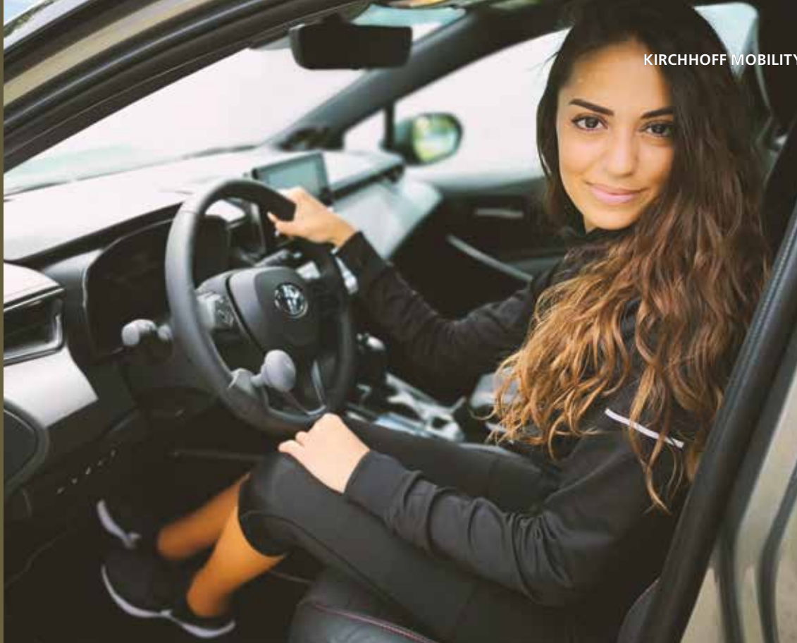
Abassia in her Toyota Corolla Hybrid with hand control Carospeed for throttle and brake, steering wheel knob Ergo and pedal cover.
