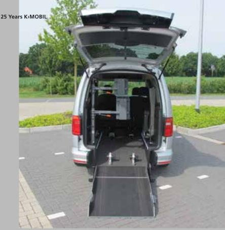
One of the core products of KIRCHHOFF Mobility: The NIVO rear cut-out kit, displayed here in the VW Caddy. Disabilityaccess conversions for various high roof station wagon models are based on this kit.
