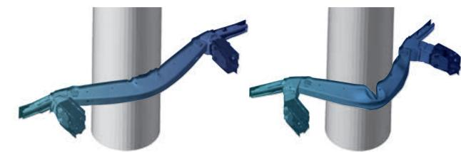
Protection of the battery comes by rigidity or flexible crash management systems for the greatest possible delay in a crash. Which variant is used, depends on the load path concept, i.e. the design of the body-in-white structure with regard to passive safety.
