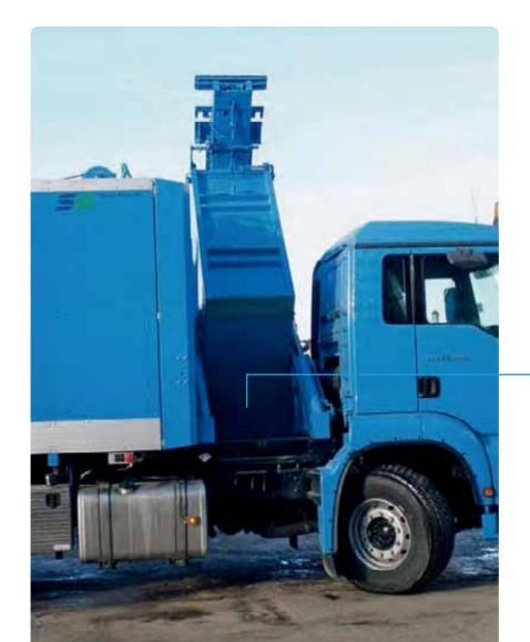
Bio or glass box in tipping position, for lateral emptying. The bio box is also available in a stainless steel version.
