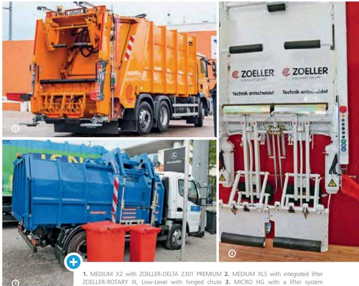
arranged on the right side 4. ZOELLER-DELTA-2307 PREMIUM, electric lifter with 24-volt motors
