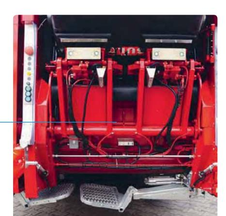
MEDIUM XLS Split with footboards that can be pneumatically extended and retracted
