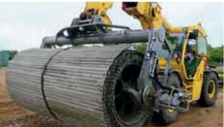
**Left:** MGMS-BD prevents vehicles from getting bogged down. **Right top:** MGMS-BD LITE, a lighter, cost-effective option. **Right down:** A standout feature of the MGMS-BD is its rotating head, allowing the system to be rotated 180 degrees so the plant can fit through smaller gaps, further aiding forces' manoeuvrability.
