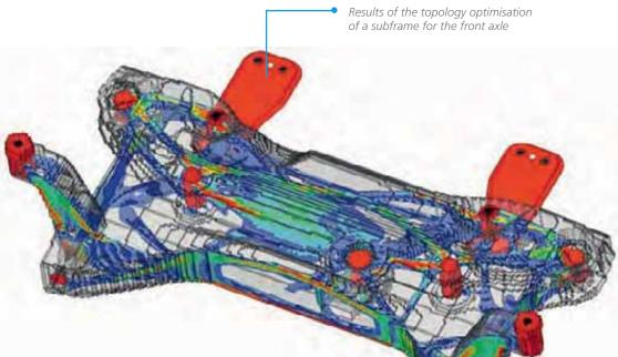
The methodology essentially consists of the following steps: Initially, the maximum available space for the components to be optimised is determined in a CAD system. Depending on the requirements, this may be the total installation space for the creation of a design for a complete assembly. Equally, subareas can be used for the optimisation of individual parts (e.g. cast nodes). The objective is to find a design that
