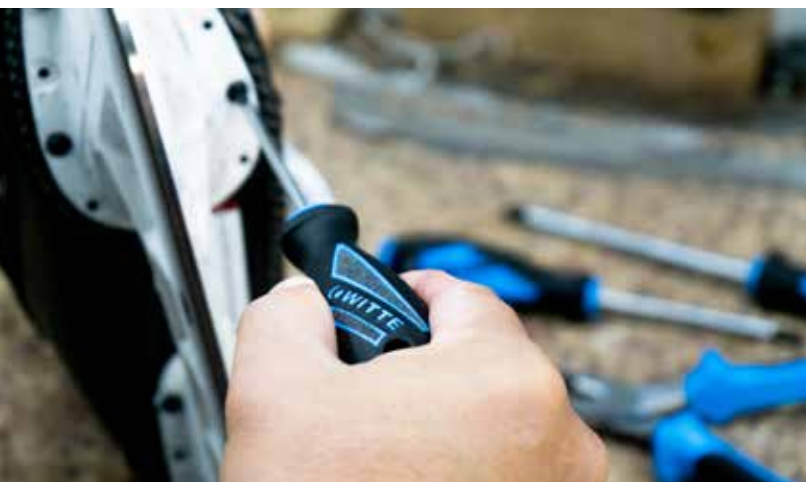
In the Roosters workshop: replacing the runner holder on an ice skate using a professional tool for professional ice hockey equipment
