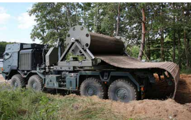
Heavy Ground Mobility System deploying M150 Trackway® to create a bridge head at Saber Strike in Poland, June 2018.
