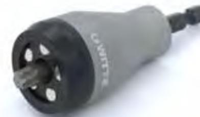
The patented screw holder is equipped with five flexibly mounted neodymium magnets that firmly fix both pan head and countersunk head screws. The retaining ring in the holder anchors interchangeable bits with drives TORX 40-50.
